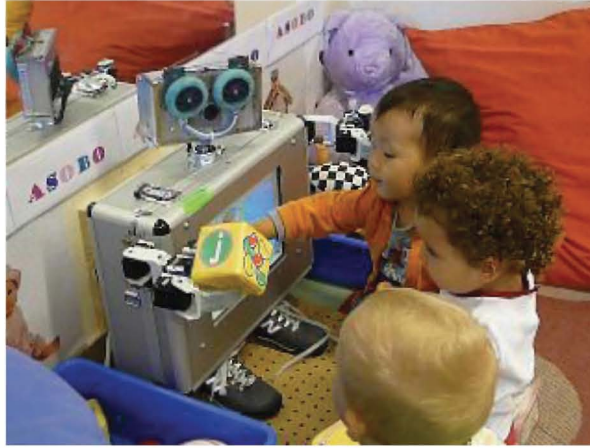
Fig. 43.8 A social robot can operate autonomously with children in a preschool setting. In this photo, toddlers play a game with the robot. One long-term goal is to engineer systems that test whether young children can learn a foreign language through interactions with a talking robot.
